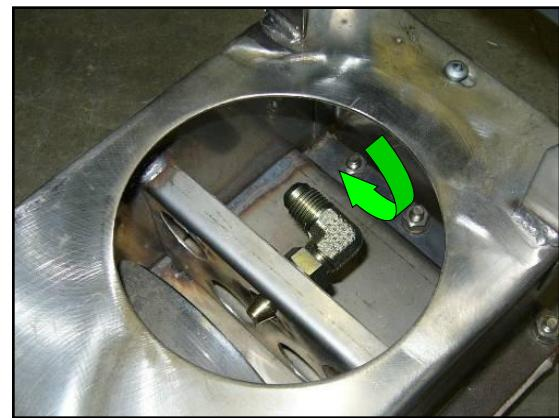
3. Use an 11/16" wrench to loosen the locking nut on the large nozzle assembly installed in the heater.
