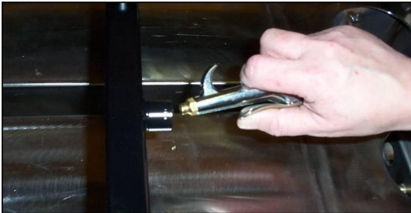
7. When all fittings have been removed, carefully clean out all teflon sealant and other debris using a fine wire brush and thoroughly blow the manifold out with compressed air
