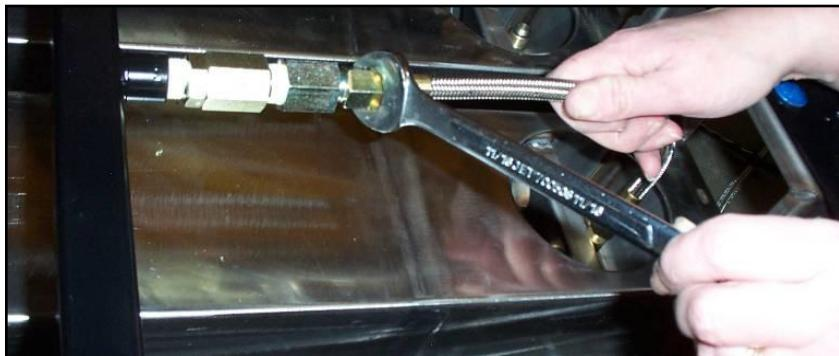
10. Then attach the other end of the hose to the Filter Assembly.
