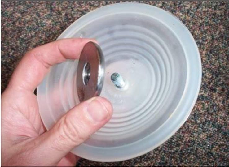
Make sure that the inner piston (shown left) is positioned with the rounded edge toward the inside of the diaphragm. Do not exceed 90 in-lbs (10.7 N-m) when securing to shaft.
