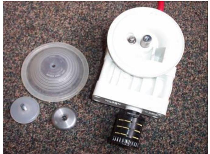
Use a 7/8" wrench and socket to remove the diaphragm from the shaft and piston. Use a vise (**with protective jaws to prevent any damage to the shaft**) to remove the diaphragm from the other side.
