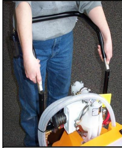
2. Connect the RSG gun to the hose and the 3 hoses to the Hopper Assembly.
