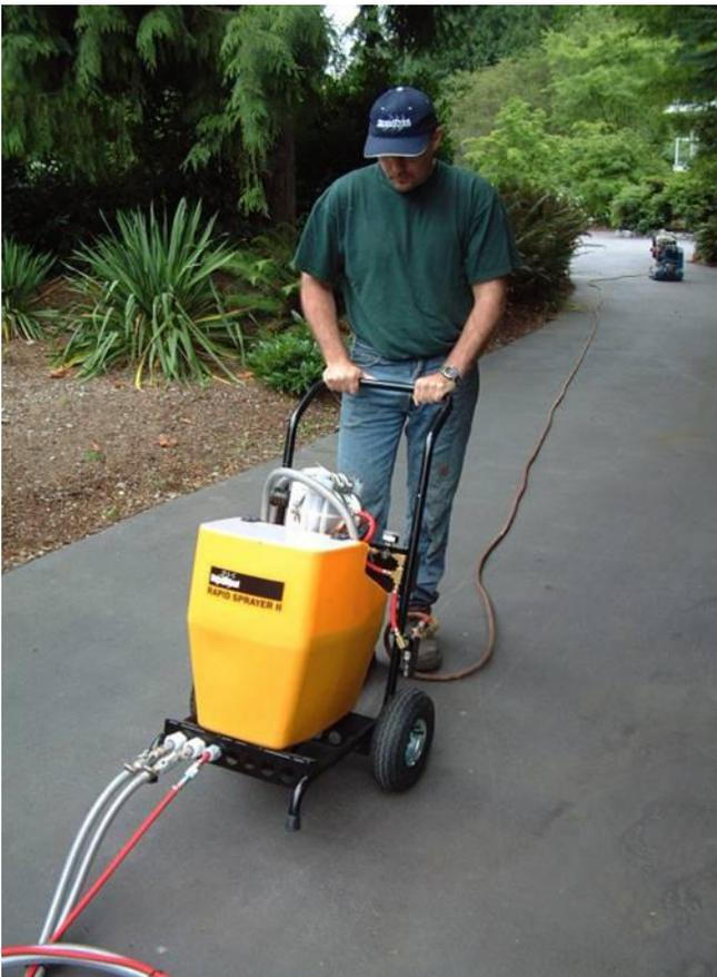
Place the compressor at the finish point of the job as shown to best keep the hoses out of the way.
