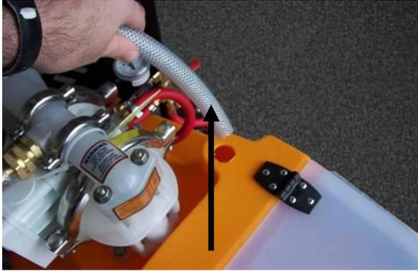
Ensure return feed hose is placed in hole at top of hopper.
