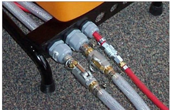
Connect the recirculation hose, discharge hose and air hose to the hopper and pump as shown
