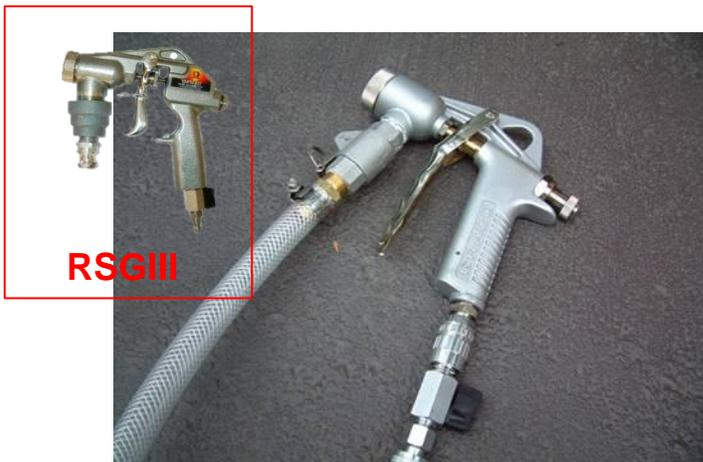
Connect the two hoses to the RSG Gun as shown
