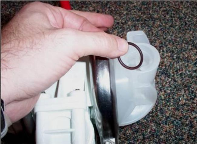
Instructions show the ball valve installation on the liquid chamber. The same applies to the discharge manifold. Insert one o-ring
