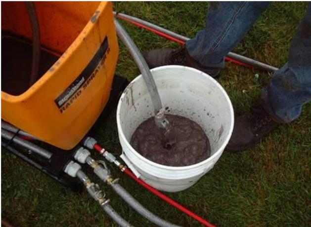
Empty out the water into buckets. Add more clean water and repeat the process until the water remains clear and the hoses are all clear of coating. Undo all cam lock couplers and clean them thoroughly to ensure a good seal on next use.
