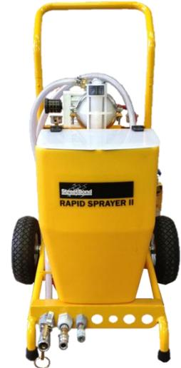
**Power Requirements:** The air supply is from a compressor (not supplied) which is capable of supplying at least 12-14 cfm (0.3 cubic meters/ min.) of continuous air at 60-80 psi. (400 – 550 atmospheres).
