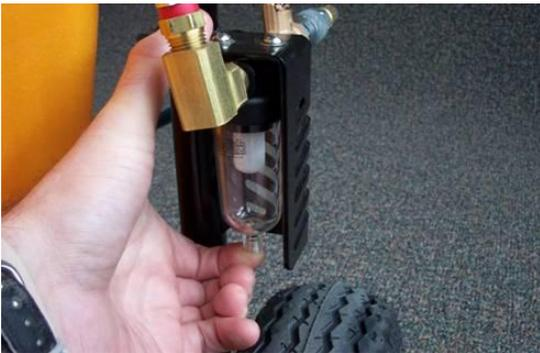
Make sure the air filter has been purged of water. To drain, press button on underside as shown.
