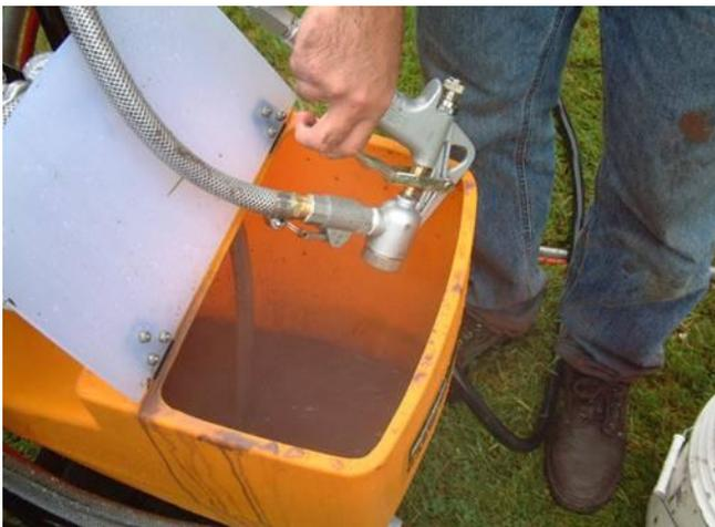
Cycle the water through the system making sure that both the gun hose and the recycle hose are thoroughly flushed of coating.
