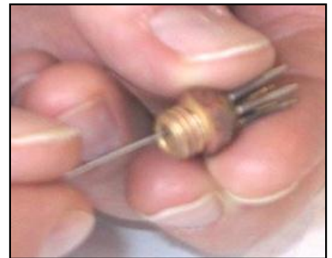
Use a 0.6mm drill to clean out each orifice stem.
