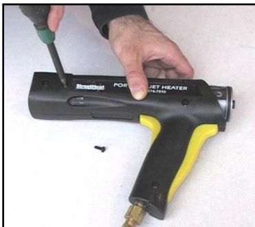
Depress button and remove tube extension and undo the 5 assembly screws.
