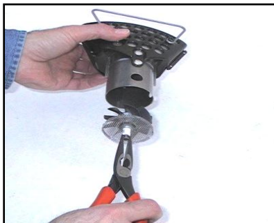
Pull spark plug, flame holder and gauze out using a pair of pliers.
