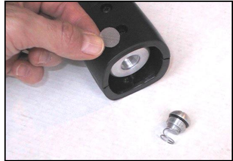
Pull out filter screen/spring assembly and clean with compressed air or replace.
