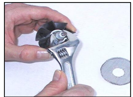
Unscrew spark plug. Note: when reinstalling gauze make sure it is snug up against the flame holder to prevent flashback.
