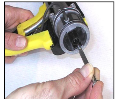
Undo contact screw which retains the cable and the contact spring (continued...)
