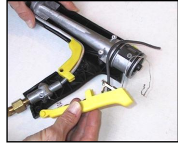
Now the trigger assembly can be removed
