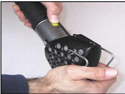
Depress button and remove the combustor assembly.
