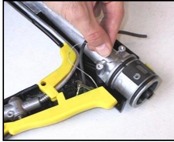
Untie and remove the ground strap.
