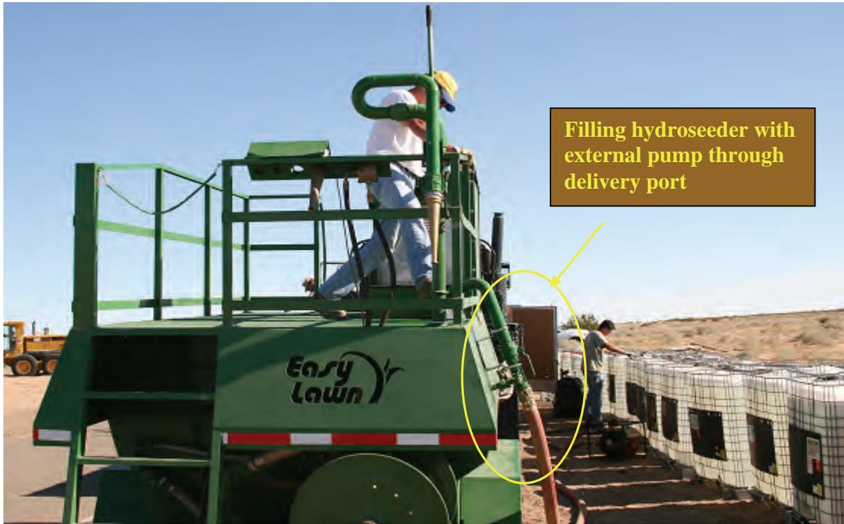
Photo 15. Filling Easy Lawn hydroseeder using external pump
