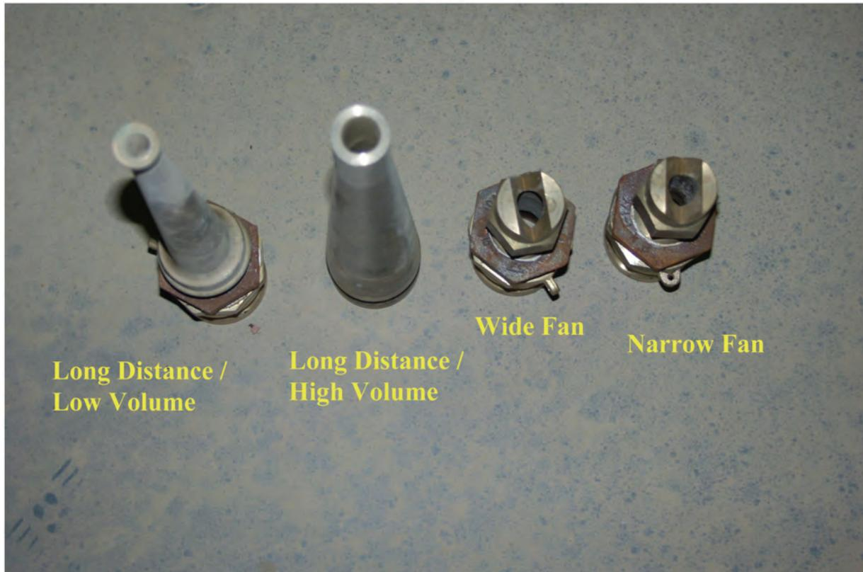
Photo 28. Spray nozzles for various spray patterns
