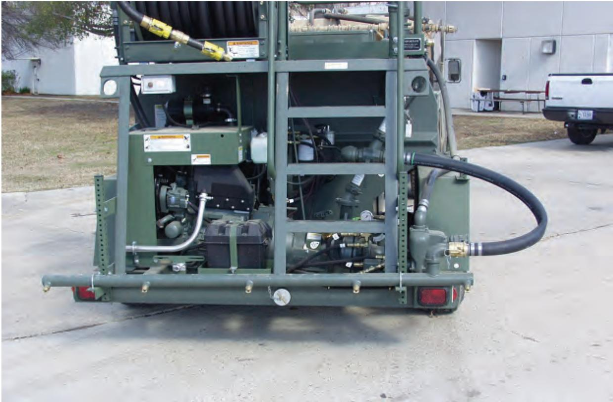
Photo 29. Distribution bar on rear of hydroseeder
