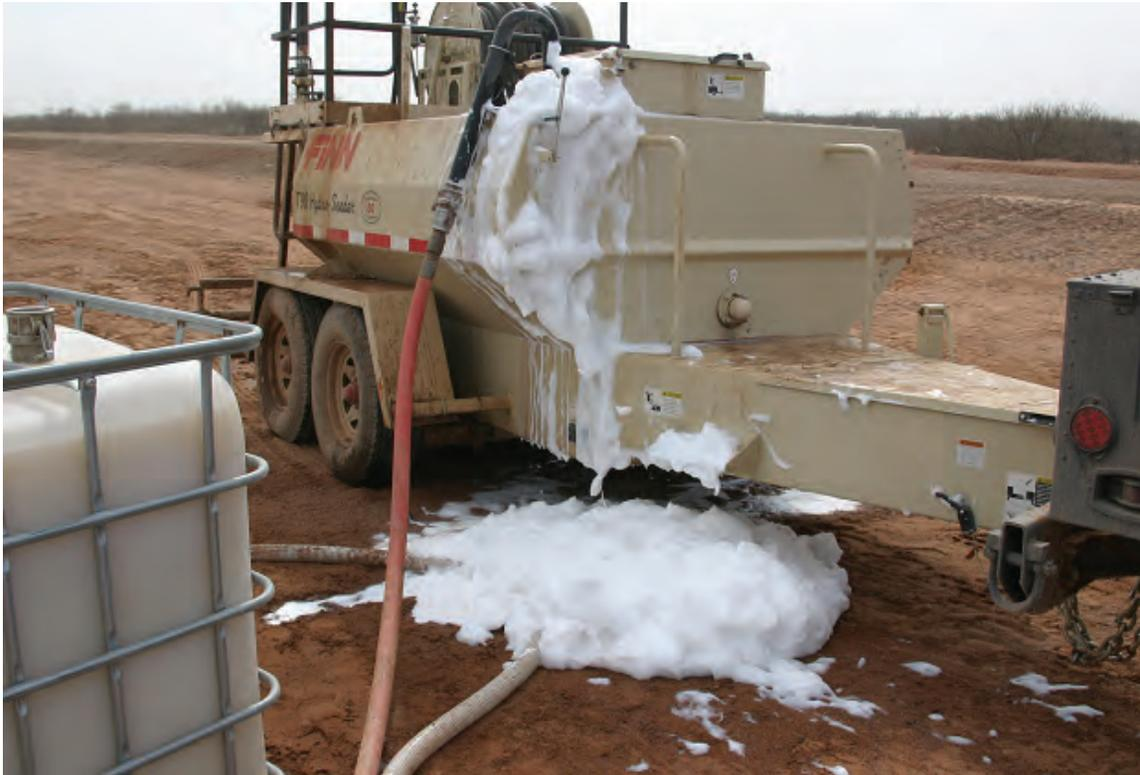
Photo 33. Excessive foaming in hydroseeder as dilution water is added to
