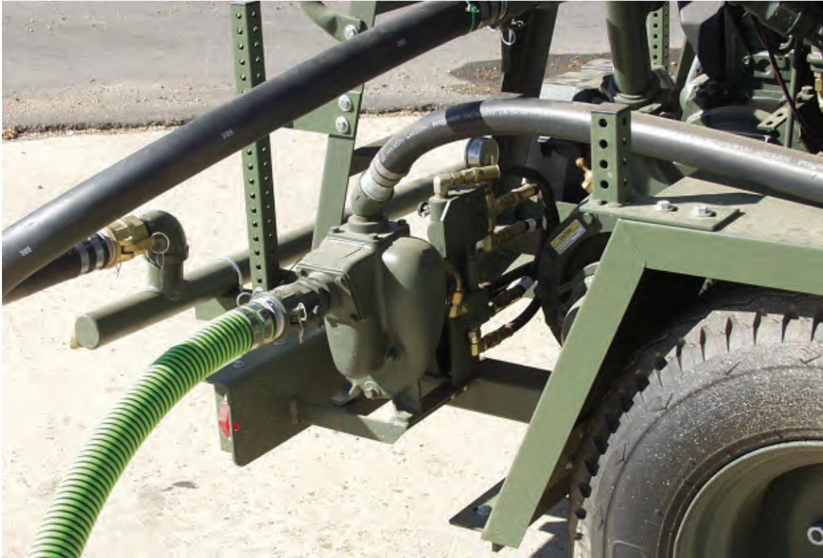
Photo 21. Filling hydroseeder from storage container using onboard hydrostatic pump
