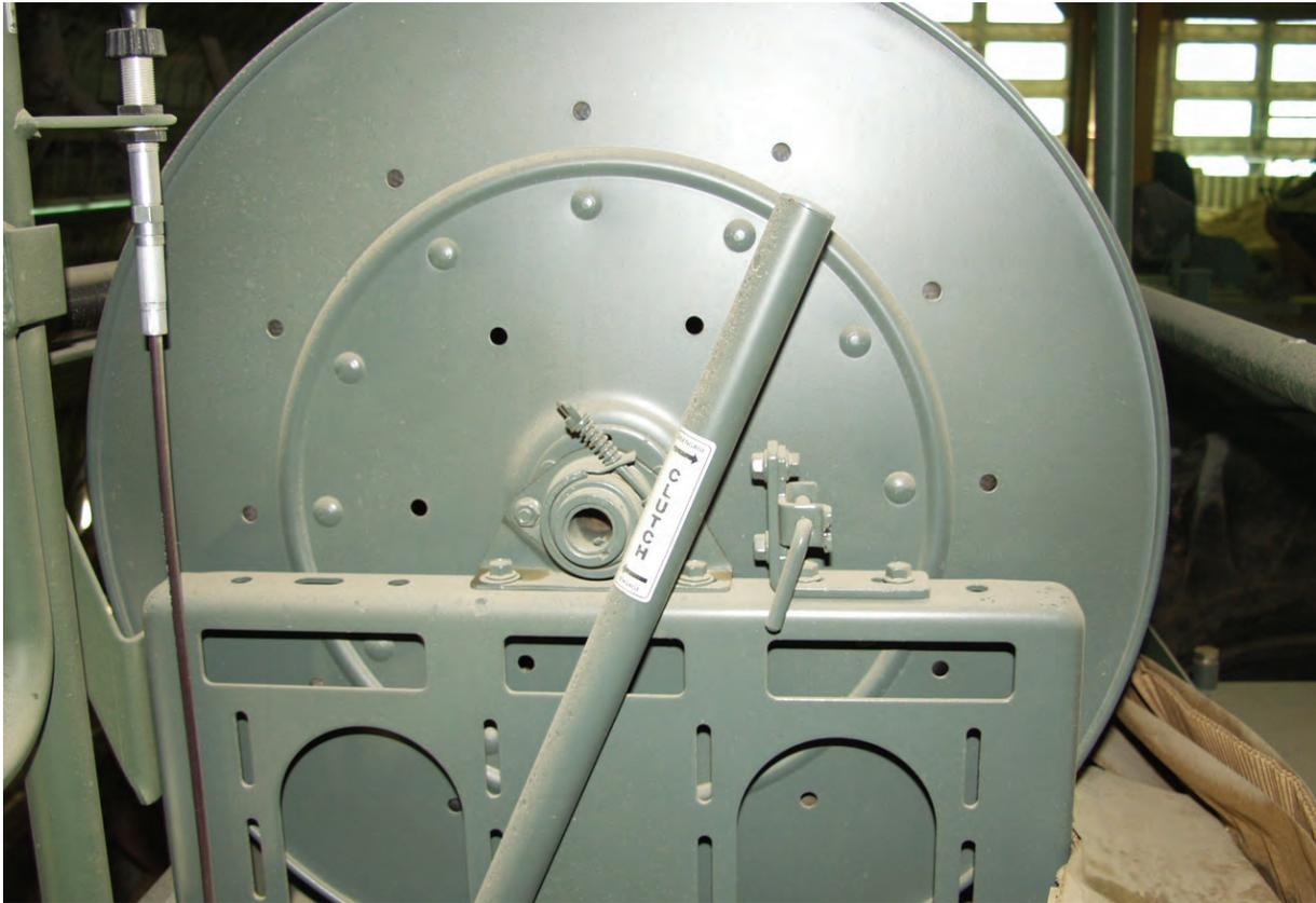
Photo 26. Clutch lever for operating pump
