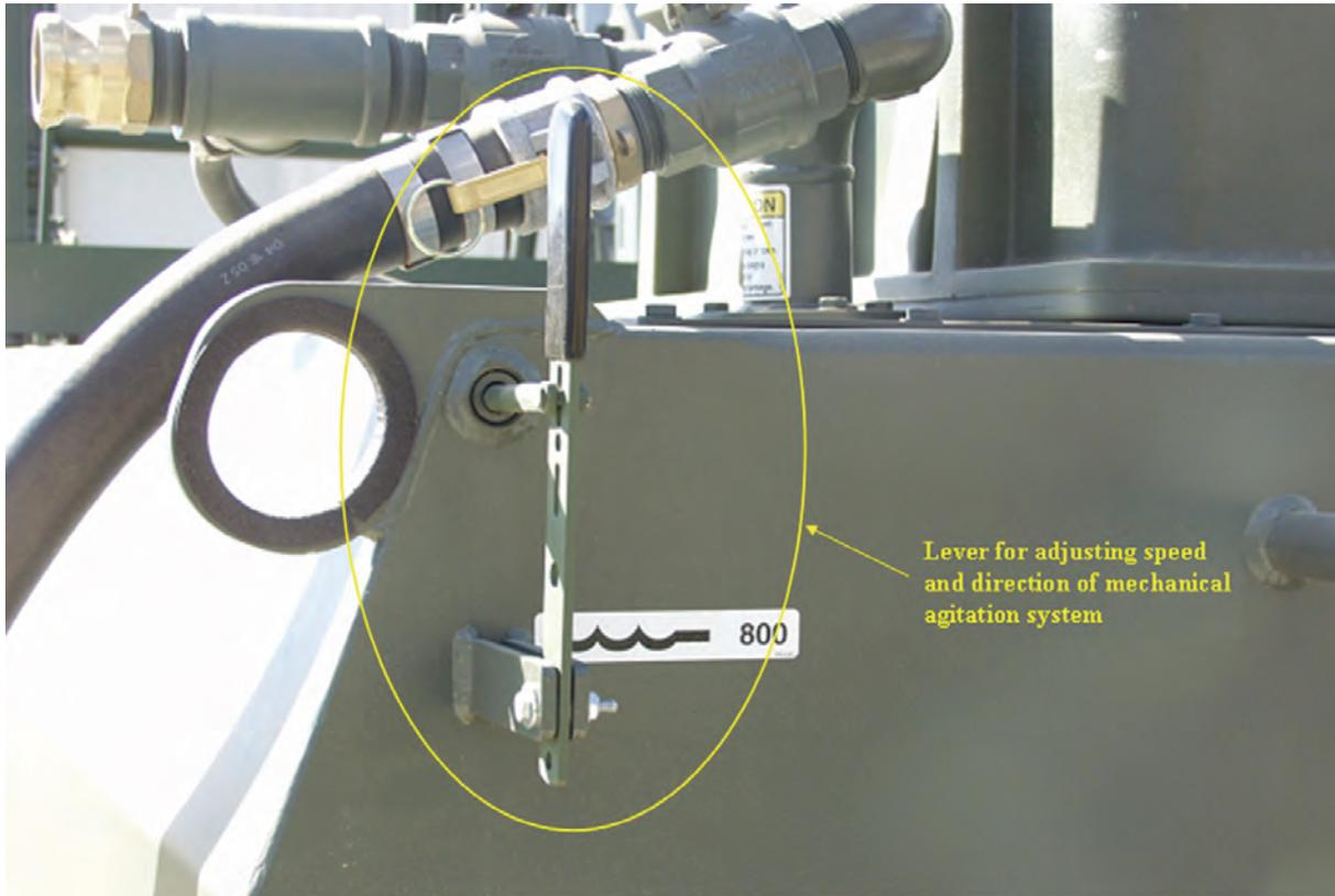
Photo 24. Lever for controlling mechanical agitation system
