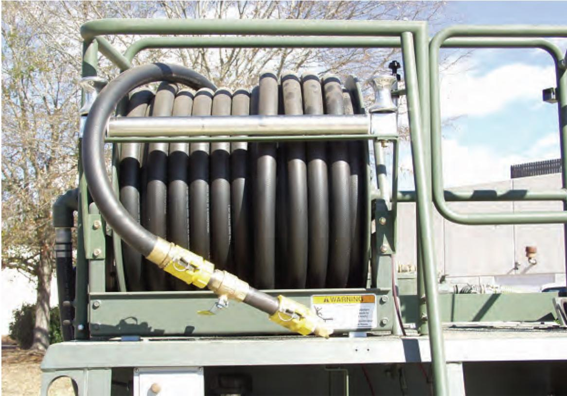
Photo 25. 200-ft hose with electric reel for multiple-use palliative distribution
