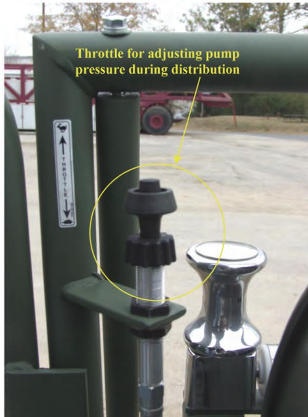
Photo 27. Engine throttle for Finn hydroseeder located by tower gun
