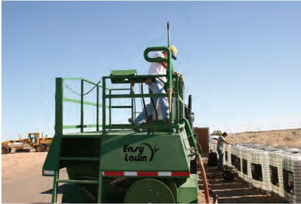
Photo 1. Filling hydroseeder with product (step *b*)
