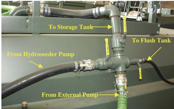
Photo 5. Multiple distribution paths for filling hydroseeder
