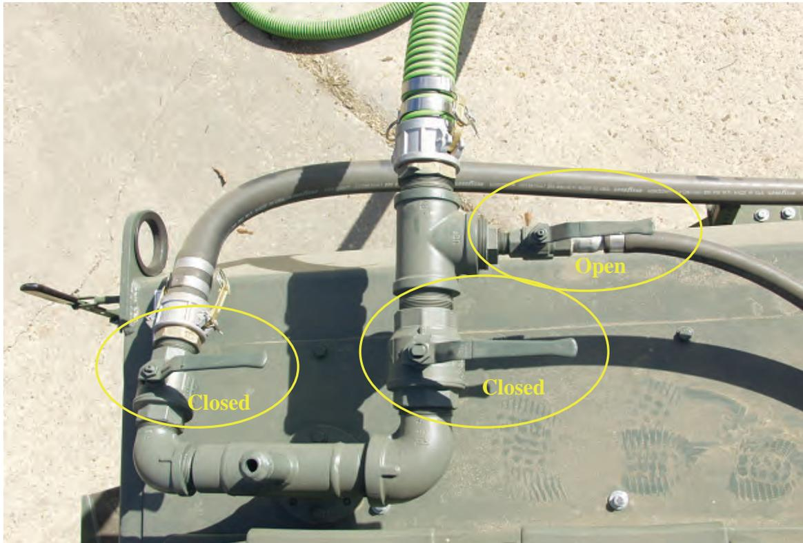
Photo 23. Filling flush tank from external water source
