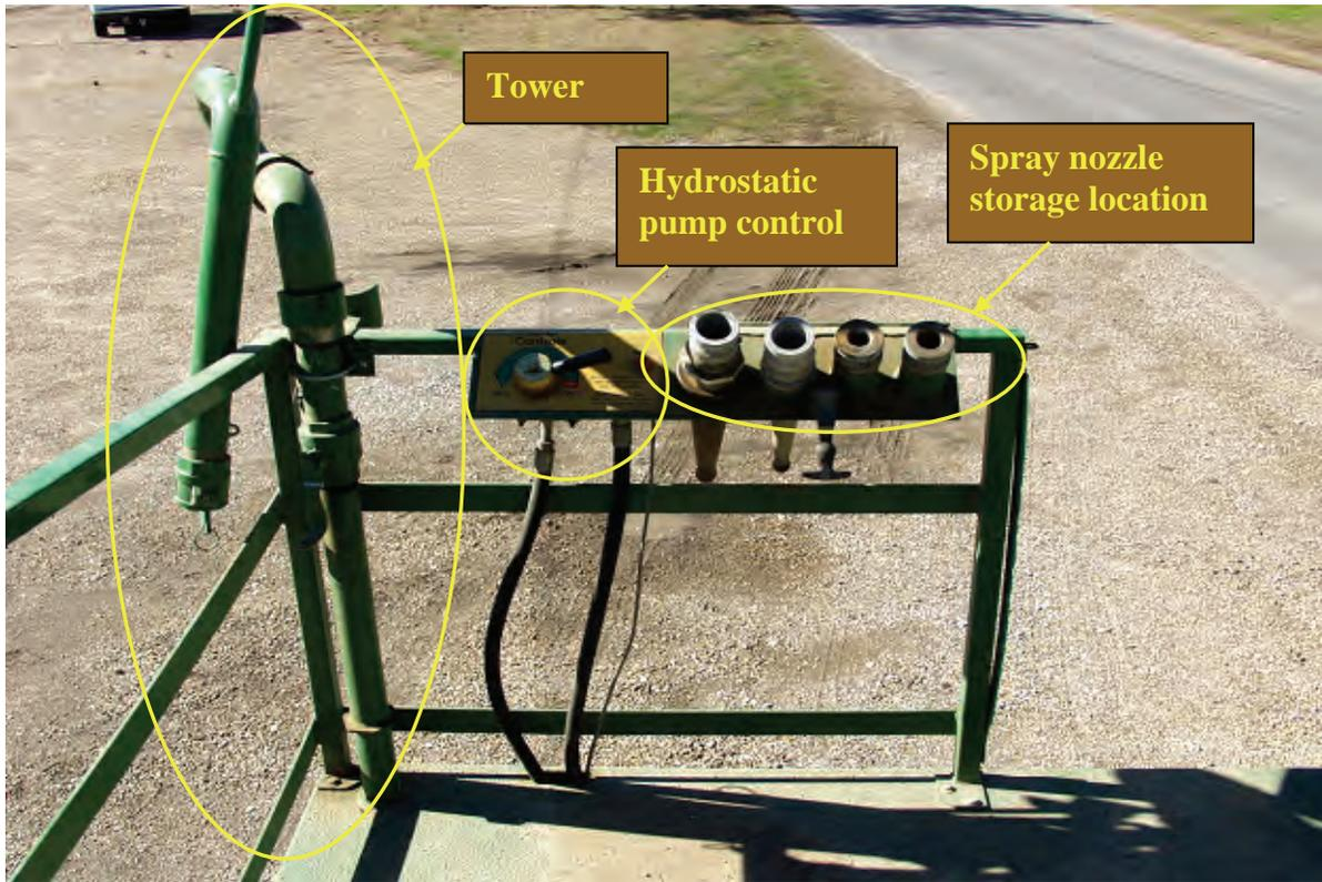
Photo 18. Control deck on Easy Lawn hydroseeder
